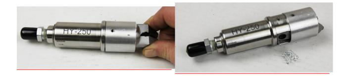
With the jaw guard and springs removed, simply <u>push</u> the center pivot pin out of the jaw body. The pinch off jaws can now be removed.
