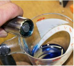
Remove the O-ring seal Remove the snap ring to separate the piston cup from the shaft. Remove the spring.
