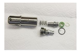
Inspect all components for wear and replace as needed. Reassemble in reverse order.
