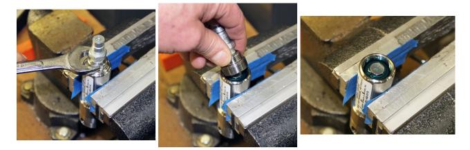
Remove the tool from the vise. <u>Place a finger on top of the shaft before emptying the oil.</u> The internal components are now loose. When the oil is drained you can now remove the internal components and spring.
