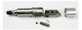
Check the rear jaw rollers and front carbide rollers for excessive wear or chipping. Replace if necessary.
