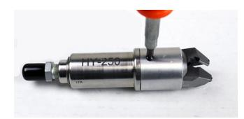
Remove small Phillips head screw at the base of the jaw guard.
